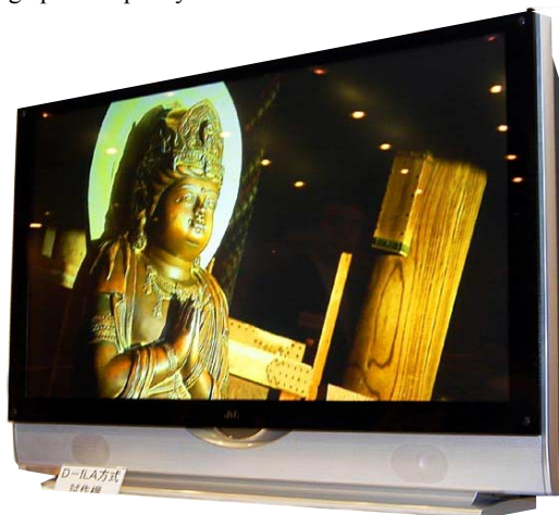
Fig. 9 Rear Projection TV model using the digital D-ILA
